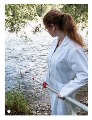
TeleScoop is a versatile sampling system with exchangeable tools for a wide range of applications. The tools (angular beaker, pendulum beaker, bottle holder, stainless steel beaker and dip net) are attached to the telescopic rod by a practical snap-in joint.
